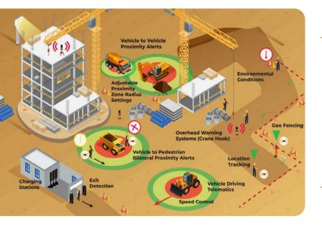
CraneGuard plays a crucial role in our Crane Safety System as a primary component. Leveraging ultrawide band (UWB) technology, it establishes a safety zone, offering the flexibility to either safeguard an area from unauthorized access by workers or provide individual alerts to workers within proximity.
